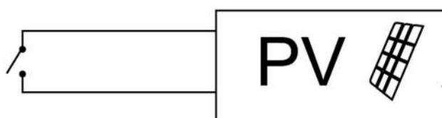
When the contact is closed, the system automatically changes to Photovoltaic mode and the heat pump and electric heater work to achieve the programmed temperature. When the contact is opened, the system returns to the previous mode.
